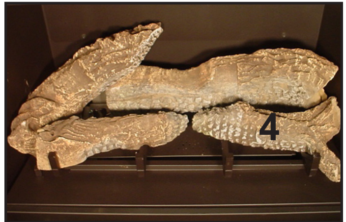
LOG #4 (SRV278-705): Position log #4 between log #1 and the locating tab on the fourth grate tine. Push its left hand side back to the locating tab as the grate tine.
